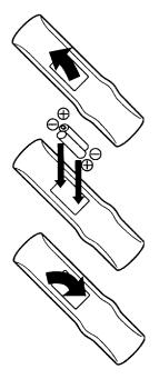
Remove the battery compartment lid on the bottom of the remote control by pressing in the tab, then lifting the lid.
